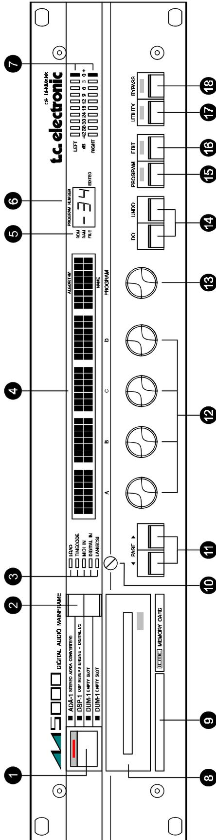
9. **MEMORY CARD SLOT** Load and stores programs into the M5000. Makes transfer of "personal" programs from one M5000 to another very easy by means of the "credit card"-like memory card.
